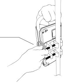
STEP 7: Tighten to secure Controller
