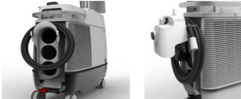
Figure 27: Power Cable on the Cable Rack
