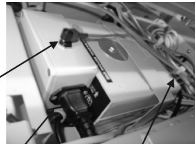
120/240V Output to Bed Control Module
