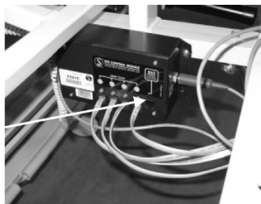
Coiled Cable from RSS Control Box to Inline Connector
