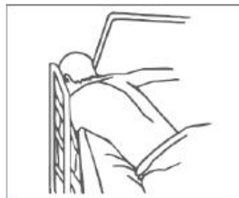
Zone 6: Between the End of the Rail and the Side Edge of the Head or Footboard
