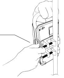
STEP 7: Tighten to secure Controller
