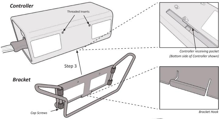
3. Firmly locate the Bracket hook into the Controller receiving pocket on the underside of the Controller. (Proper locating is critical for Step 4.)
