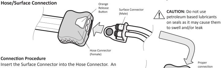
audible "click" can be heard once the Connectors are fully seated. Confirm Connector seating with a slight pull.
