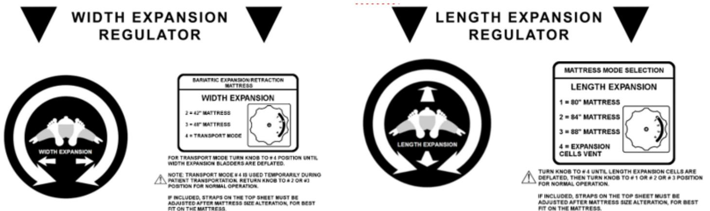
1. To inflate mattress to 42" in width, rotate the valve selector to position #2.
