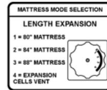
TURN KNOB TO # 4 UNTIL LENGTH EXPANSION CELLS ARE DEFLATED, THEN TURN KNOB TO # 1 OR # 2 OR # 3 POSITION FOR NORMAL OPERATION.
