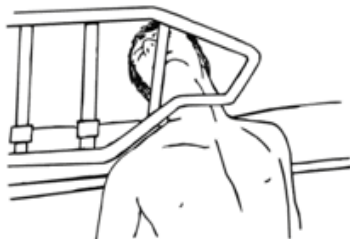
Entrapment under the bed rail at the ends of the bed rail
