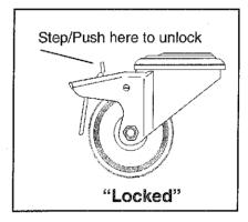
The locking function holds the bed motionless when the bed is parked. Lock all casters when transferring the patient to and from a bed. Casters are the individually locking type. For stability when parking the bed, the casters should be positioned as shown on page 14.
