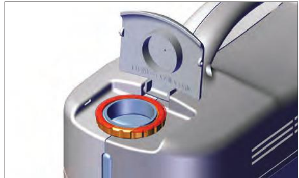
Figure 23 - Step 2 Install reservoir collar
