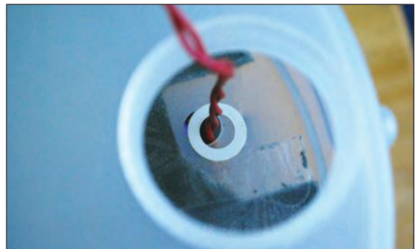
Figure 51 - Thread connector and wires through reservoir
