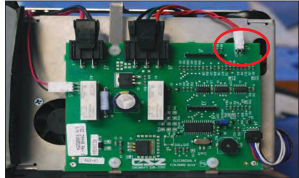
Figure 46 - Step 3 Disconnect J7
