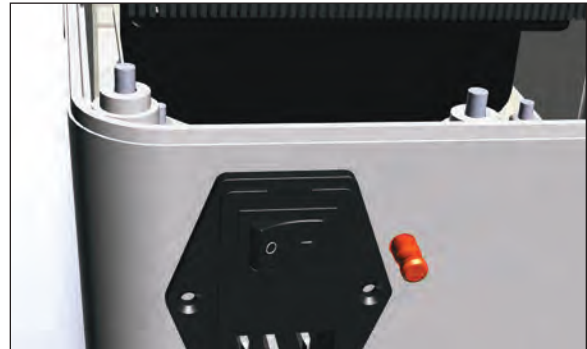
Figure 38 - Step 1 Insert stud
