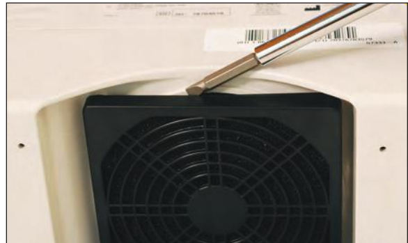
Figure 5 - Step 2 Pry off retainer
