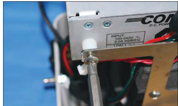
Figure 114 - Step 4 Unscrew power supply from front bracket
