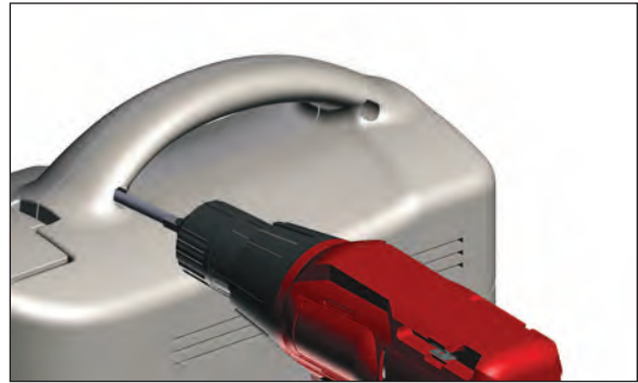
Figure 25 - Step 4 Install two handle screws
