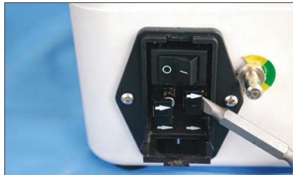
Figure 93 - Step 2 Match arrow direction
