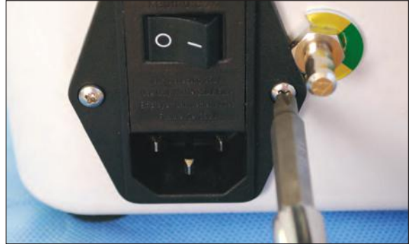
Figure 101 - Step 2 Install power inlet
