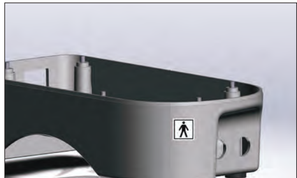
Figure 34 - Step 2 Apply the BF label
