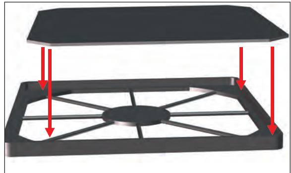
Figure 153 - Step 2 Place filter into retainer
