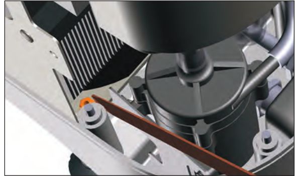
Figure 151 - Step 5 Hold Keps nut #4
