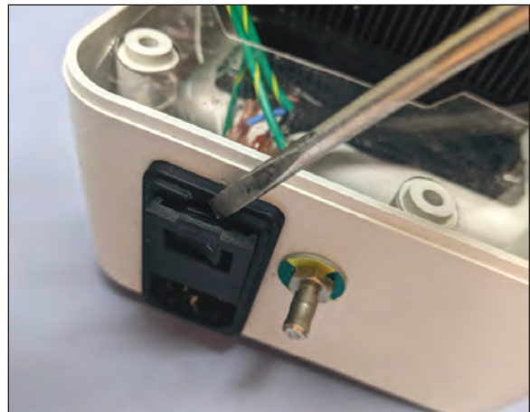
Figure 90 - Step 2 Open fuse door
