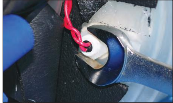
Figure 52 - Step 4 Secure float switch mounting nut
