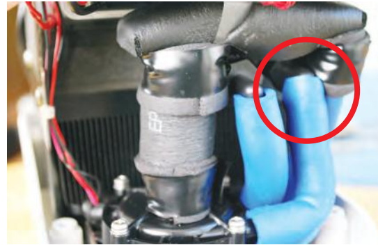
Figure 67 - Step 8 Remove inlet tubing
