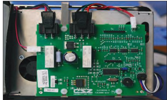
Figure 55 - Step 7 Attach connector to J7
