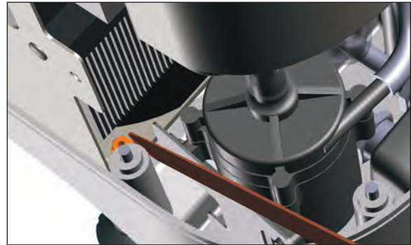
Figure 147 - Step 9 Remove Keps nut #4
