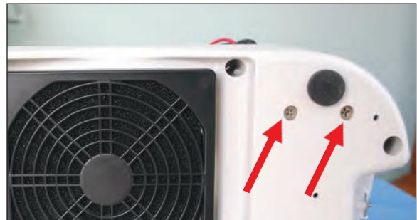
Figure 66 - Step 6 Unscrew pump bracket from base enclosure
