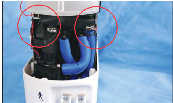
Figure 58 - Step 1 connect tubing to reservoir with clamps
