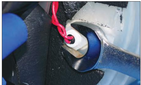
Figure 48 - Step 5 Unscrew float switch mounting nut
