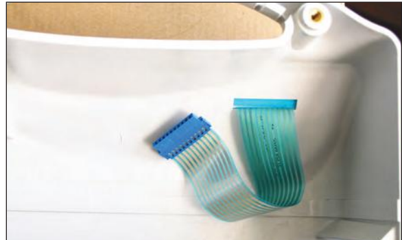
Figure 44 - Step 1 Thread cable through slot
