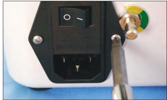
Figure 99 - Step 7 Remove retaining screws
