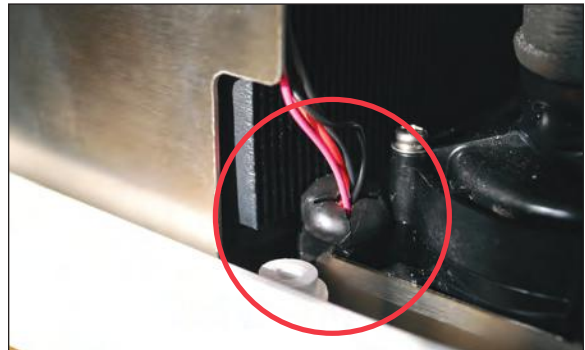
Figure 98 - Step 6 Remove suppressor
