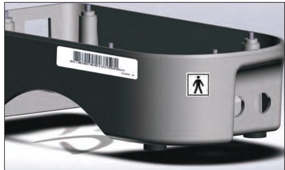
Figure 35 - Step 3 Apply the GTIN label
