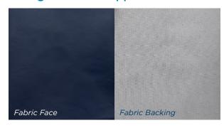
**Highly chemically resistant fabrics** withstand harsh cleaning protocols and help maintain a waterproof covering (photos: 10 days in bleach).
