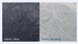
**Most top cover fabrics** lose their waterproofing when exposed to disinfecting chemicals—allowing for fluid ingress (photos: 5 days in bleach).
