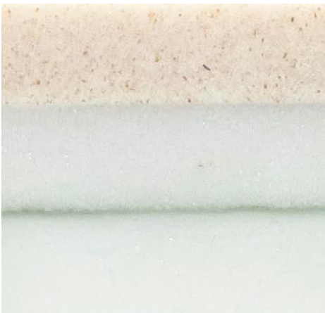
Three layers and three zones of foam for targeted pressure redistribution
