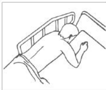
Zone 3: Between the Rail and the Mattress
