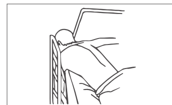
Zone 6: Between the end of the rail and the side edge of the head or footboard
