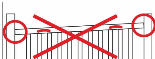
Fig. Incorrectly locked siderail
