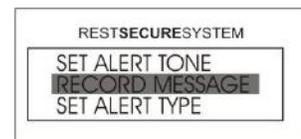
3. Press and hold the ENTER button until the user hears a series of beeps. With the ENTER button still pressed, the user may begin to record a message by speaking directly into the microphone. The message can be recorded for a maximum length of 15 seconds. When the recording is finished, release the ENTER button and follow the on-screen prompts.
