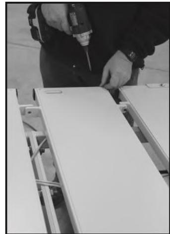
4. Locate the 3 – 5/8” bolts, washers and nuts. Place the bolt and washer together, then insert through the head section and then through the foot section of the bed. Add the washer and Nylock nut to complete the bed frame assembly. Secure tightly using 15/16” wrenches.
