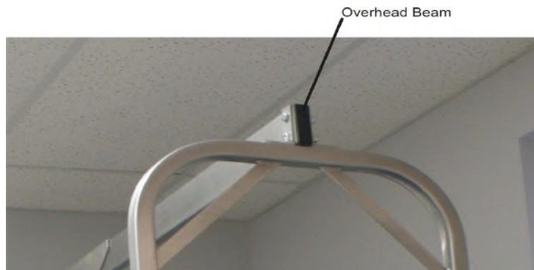
4. Attach the sliding saddle to the overhead beam. Move the saddle until the pin is secured into one of the holes on the overhead beam.
