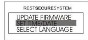
3. Using the UP or DOWN arrow, the user can set the hours and then press ENTER. The time must be set in 24-hour clock. (13:00 = 1:00 pm)
