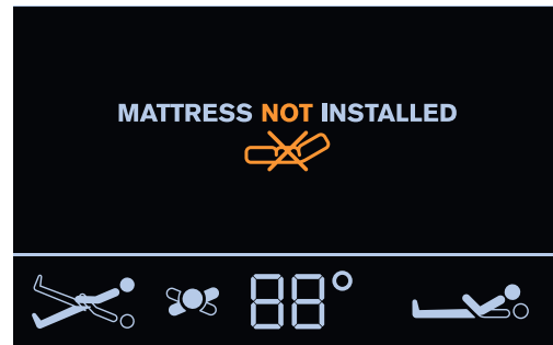
Fig. Mattress Not Installed Screen
