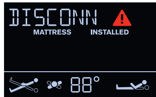
Fig. DISCONNECTED AIR PIPES
