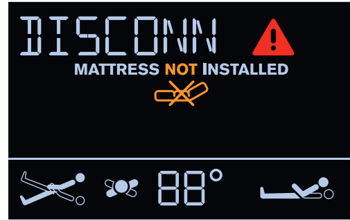
Fig. PUMP DISCONNECTED
